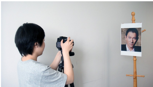
Figure 8. The self-timer scenario in which a picture board was used as a stand-in to allow the camera to autofocus.
