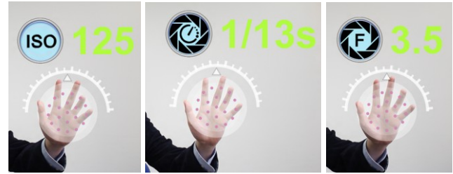
Figure 7. Value adjusting interface. Perform circling gesture inside the tracking point circle to adjust the value. The semicircular dial above will rotate according to gestures in clockwise/counter-clockwise motions. The parameters adjusted in the image from left to right are aperture, shutter speed, and ISO.
