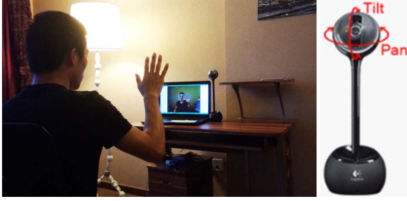
Fig. 6. The self-portrait system, including a pan-and-tilt camera and notebook computer. Gestures are used to control camera functions, such as pan, tilt and shutter trigger.
