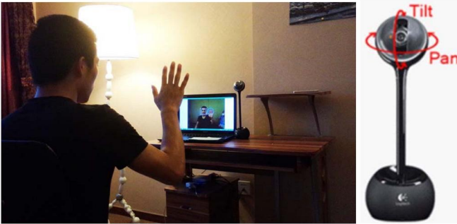
Figure 5. PTZ camera selfie system. Hand gestures are used to control camera functions. The figure is used with permission from IEEE license (Chu et al., 2017b).
