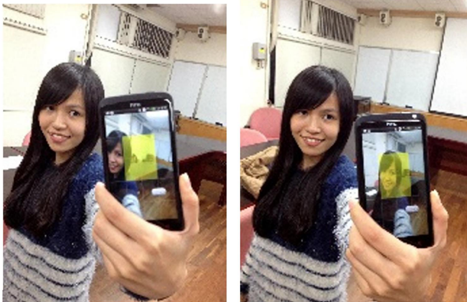
Figure 11. Yes, Right There! Prevent faces from being cut out of the camera frame by giving suggestions to users until they are in a suitable position in the frame. The figure is used with permission from authors (Lo et al., 2013b).
