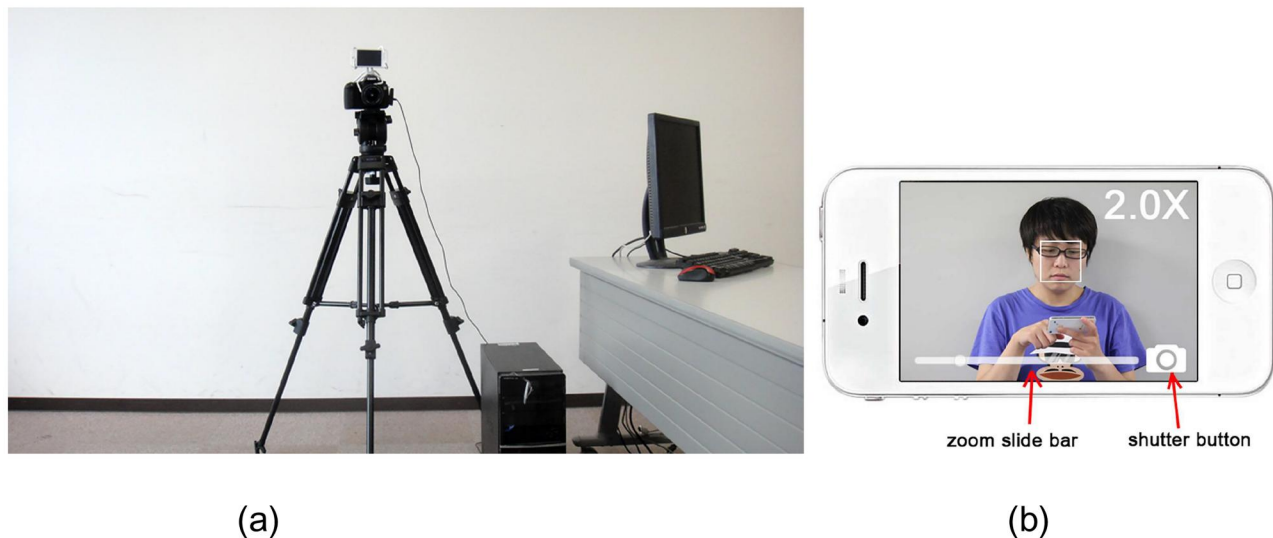
Figure 9. Using a smartphone as the remote controller to preview the frame of the DSLR camera. (a) Selfie system; (b) smartphone as remote controller. The figure is used with permission from authors (Chu & Tanaka, 2013a).
